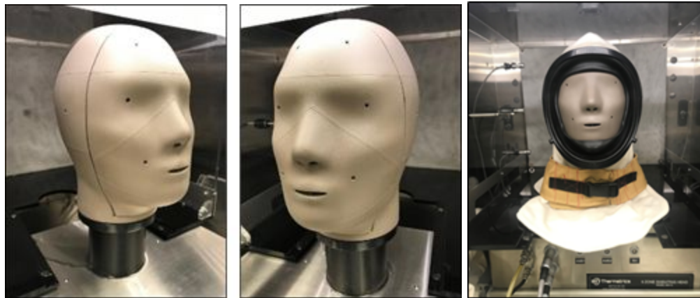
Figure 1: Sweating manikin headform, dressed in a Nomex hood for testing
